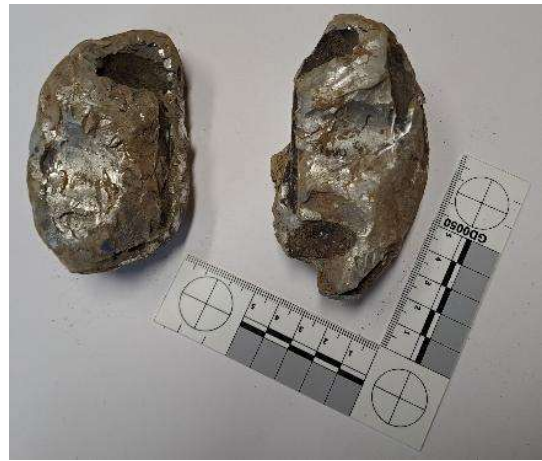
Fig. 9 – Deformed piston parts from the engine
