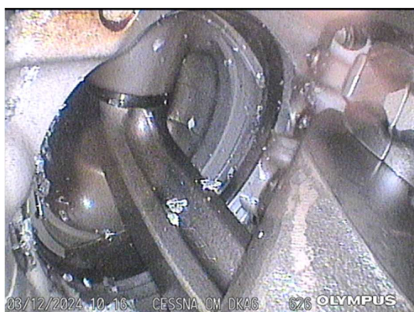
View of condition of connecting rod and piston at piston pin location in cylinder #6
