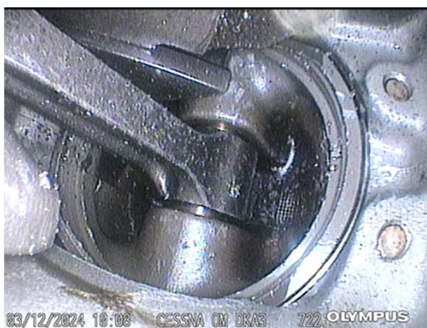
Detailed view of condition of connecting rod and piston in cylinder #3
