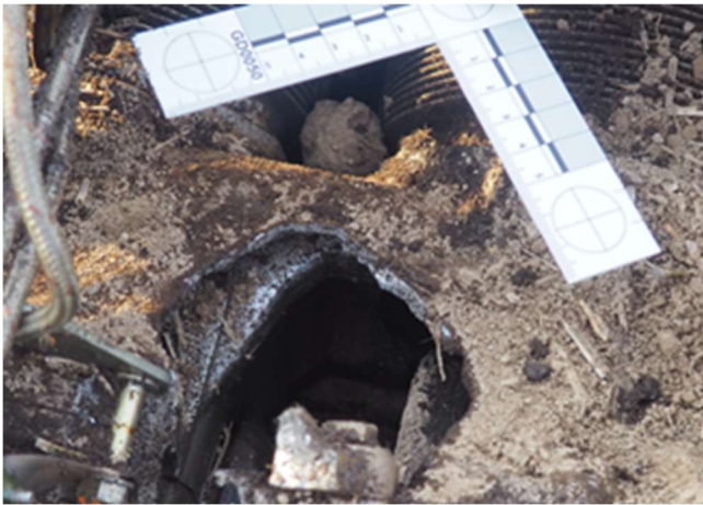
Fig. 8 – Punctured hole in the upper side of the engine
