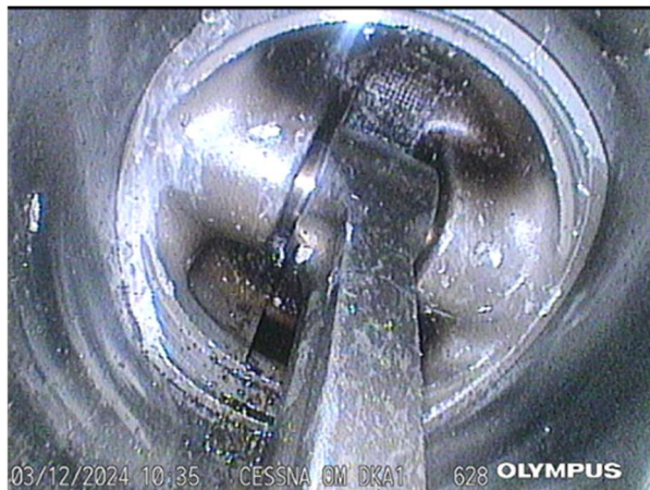
Condition of connecting rod and piston underside in cylinder #1
