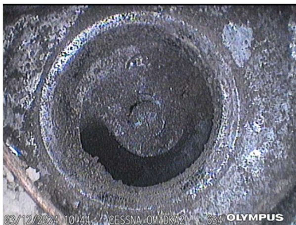
Detailed view of condition of exhaust valve opening in cylinder #2
