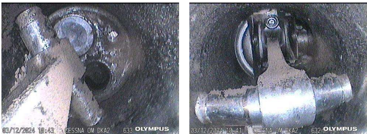
Fig. 10 – Missing exhaust valve head and piston in cylinder 2
