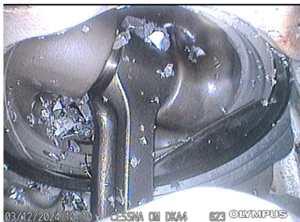
Detailed view of condition of connecting rod, piston at piston pin location and metal fragments in cylinder #4
