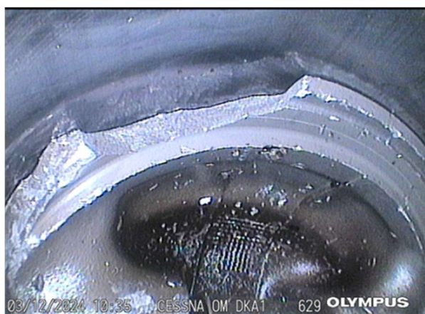
Detail of condition of connecting rod and fracture on bottom of piston in cylinder #1
