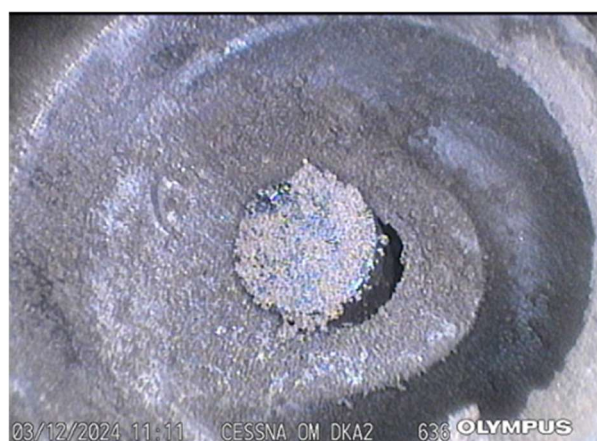
Detailed view of condition of exhaust valve bore in cylinder #2
