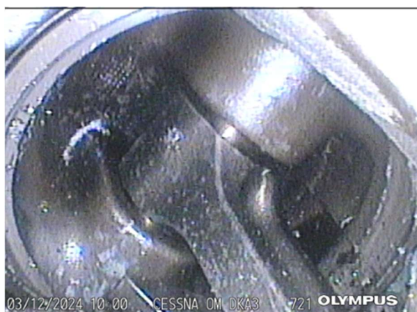
Detailed view of condition of connecting rod and piston at piston pin location in cylinder #3
